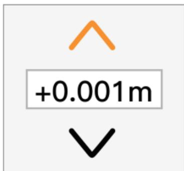
The self-calibration function is mainly used to correct data. When the deviation occurs when the user measures the distance, the function can be used to correct the distance, the correction range: -0.009~0.009m. For example, if the user thinks that the value is larger by 2mm, the value can be adjusted to -0.002m to compensate 2mm; On the contrary, if it is 2mm smaller, it is adjusted to 0.002m. The operation is as follows:
