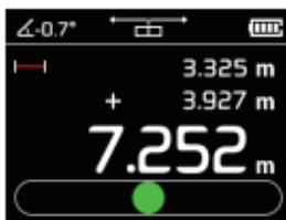
When measuring again, the instrument will automatically add up the data and sum it up
