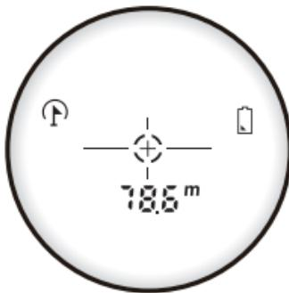
Flagpole locking function is used to measure signal towers, telegraph poles and other slender targets.
